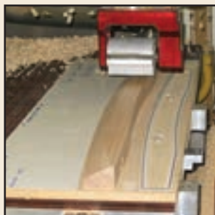
shaping with cutting knives
