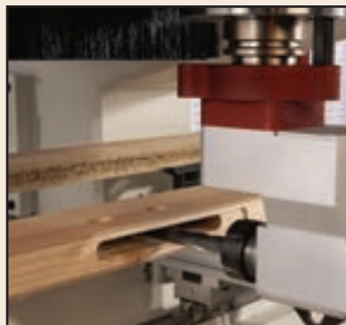
Mortising a lockset recess
