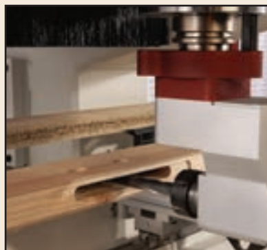
Mortising a lockset recess
